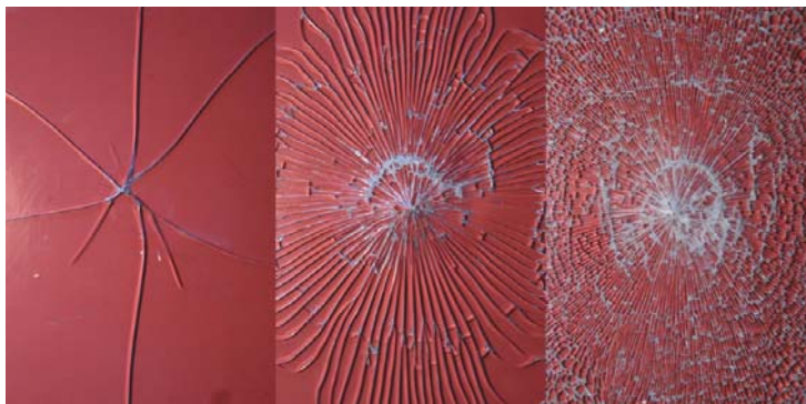
Figure 2: Form of glass breakage. From left, annealed , heat strengthened, toughened [6].
